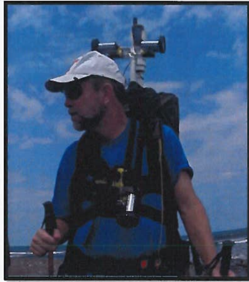
Figure 4: Dr. Parham using Backpack HDSS on Iao Stream, Maui. The GPS-linked video cameras are image stabilized to dampen the bounces associated with walking in a stream.
